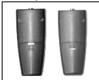
Figure 1- 7 Moving the battery door sliding tab
