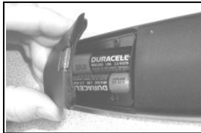
Figure 1- 9 Re-inserting the battery door
