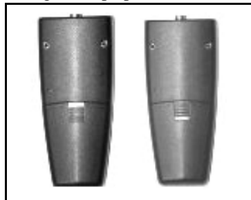
Figure 1- 10 Locking the battery door
